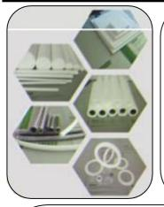
(Polytetrafluoroethylene) PTFE has excellent resistance to the majority of chemicals and solvents and is capable of operating at high and low temperatures. It also has a very low coefficient of friction and is commonly used in food contact applications. PTFE provides good thermal stability and has good electrical properties, but is not suitable for wear application and is difficult to bond.
