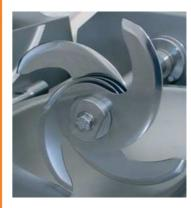
The knife shaft is driven by v-belts.
